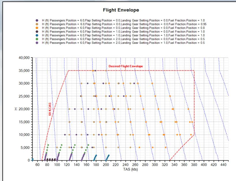
Full flight envelope covering flaps, landing gear and fuel fractions to...
