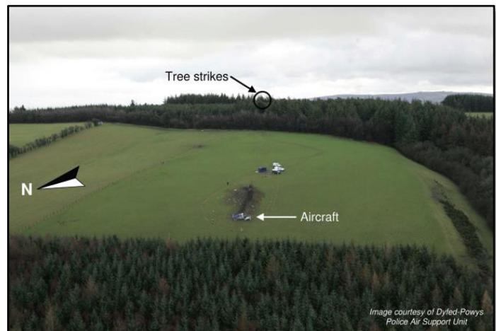
A series of dynamic scenarios were constructed based on the reported altitude, flight path, airspeed and wind/weather conditions. The j2 software was used to introduce a point force acting on the leading edge of the wing as it struck the tree, resulting in the instantaneous loss of  $\frac{1}{3}$ <sup>rd</sup> of the outboard left wing. The software automatically calculated the resulting changes in aerodynamic characteristics.
